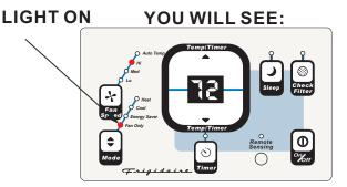
Note: Use this function only when cooling is not desired, such as for room air circulation. You can choose any fan speed you prefer, EXCEPT AUTO FAN.
